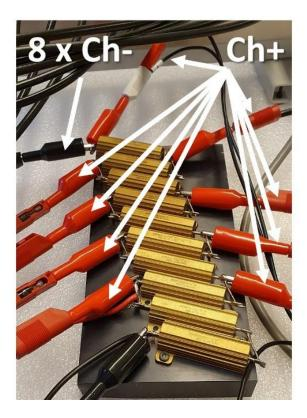
This connection should result in 9 impedance signals of 10 Ohm and 1 Ohm – 8 Ohm respectively.
