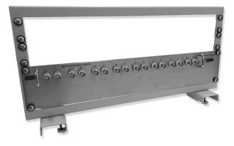
The module is powered from a 5V DC power supply and connects to the 15pin subD connector of the peripheral port. At the front the StackAnalyser has 8 channels, each with 2 BNC connectors for the Chand Ch+ respectively. In this case, each of the 16 BNCs has its own BNC to 4mm banana cable.
