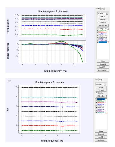
Scan 1 is the primary signal, i.e. the cell cable. Scan 2 is Ch1 of the StackAnalyser Scan 3 is Ch2 of the StackAnalyser etc.
