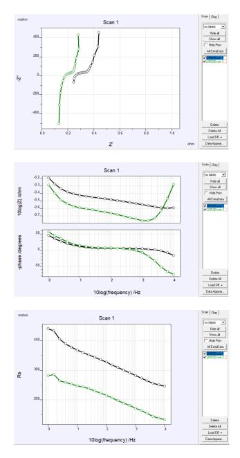
In the measurement results, the different impedances can clearly be distinguished between the total (black line, scan1) and the AA-battery to the left (green line, scan2).
