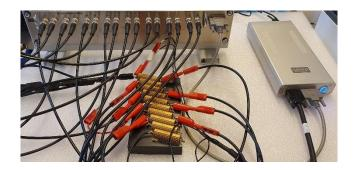
The WE+S of the cell cable are connected to the resistor to the left, the CE+RE of the cell cable are connected to the resistor to the right.
