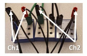
This connection should result in 3 impedance signals of 3kOhm, 1kOhm and 2kOhm respectively.
