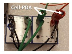
This connection should result in 2 impedance signals of 2kOhm and 1kOhm respectively.
