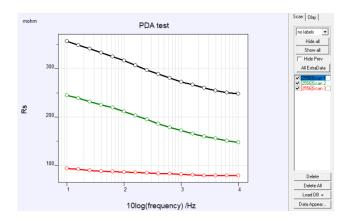
In the measurement results, the different impedances can clearly be distinguished of the total (black line, scan1), battery1 (green line, scan2) and battery2 (red line, scan 3).
