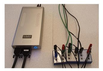
The CE+RE of the cell cable are connected to the TestCell1 to the left, the WE+S of the cell cable are connected to the Testcell1 to the right.
