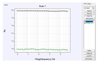
Scan 1 (black) is the primary signal, i.e. the cell cable. Scan 2 (green) is Cell-PDA signal
