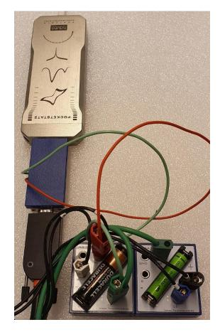
The WE+S are connected to the + of the battery to the left. The CE+RE are connected to the - of the battery to the right. The cell cable will thus measure the impedance of the total (= the two batteries in series).
